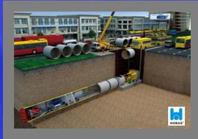
**Hypothesis** "Trenchless installation method of sewer pipe is a **better environmental choice** in regard to climate change than open-cut".
